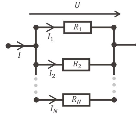
$$\frac{1}{R_{\text{eq}}} = \sum_{k=1}^N \frac{1}{R_k} \quad / \quad G_{\text{eq}} = \sum_{k=1}^N G_k$$
