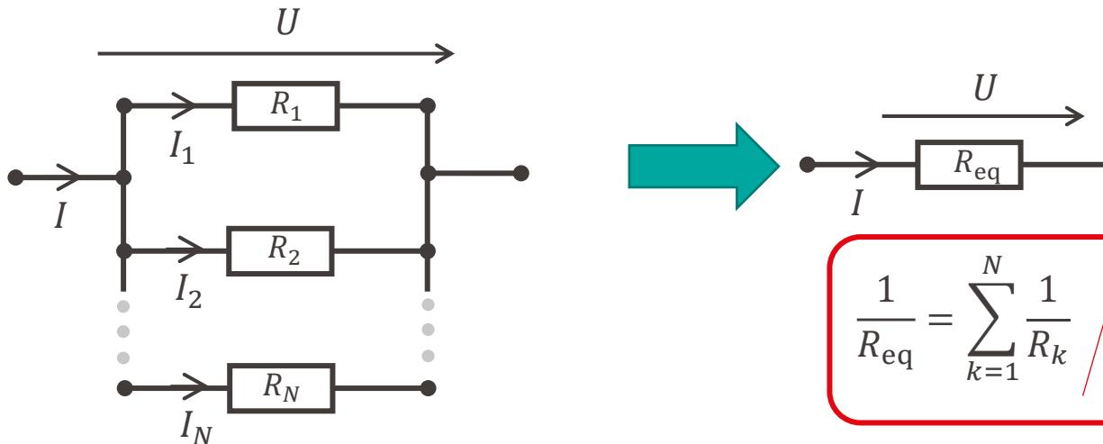
$$\frac{1}{R_{\text{eq}}} = \sum_{k=1}^N \frac{1}{R_k} \quad / \quad G_{\text{eq}} = \sum_{k=1}^N G_k$$
