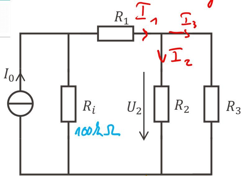
$$\begin{aligned}I_0 &= 110 \mu\text{A} \\R_i &= 100 \text{ k}\Omega \\R_1 &= 1.25 \text{ k}\Omega \\R_2 &= 10 \text{ k}\Omega \\R_3 &= 10 \text{ k}\Omega\end{aligned}$$
