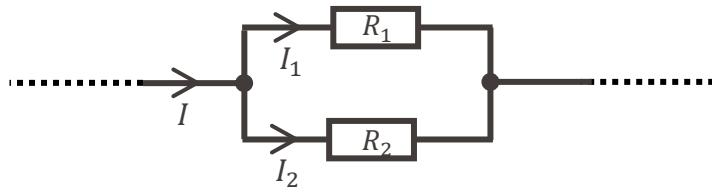
$$I_1 = \frac{R_2}{R_1 + R_2} I$$
