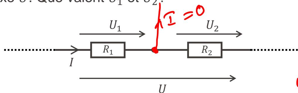
$$U_1 = R_1 I \quad / \quad U_2 = R_2 I$$
