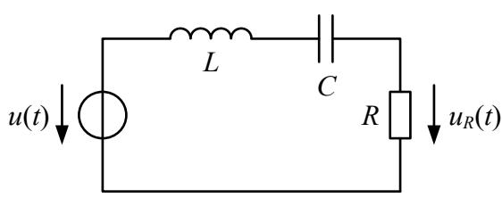
$$\begin{aligned}R &= 1 \text{ k}\Omega \\L &= 10 \text{ mH} \\C &= 10 \text{ nF} \\u(t) &= \hat{U} \sin(2\pi ft) \\u_R(t) &= \hat{U}_R \sin(2\pi ft + \varphi)\end{aligned}$$
