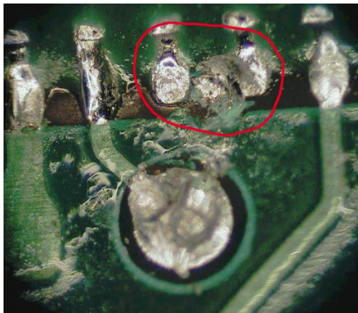
poor soldering (manufacturing)...
