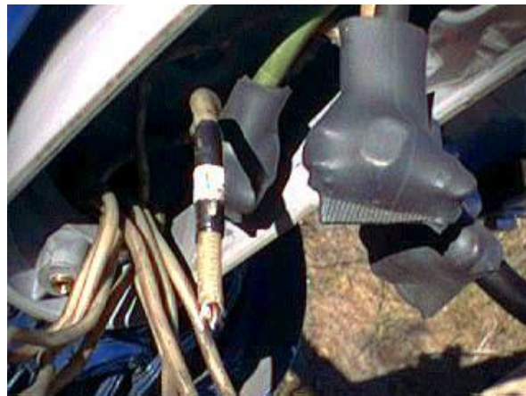
broken wire... (vibrations)
