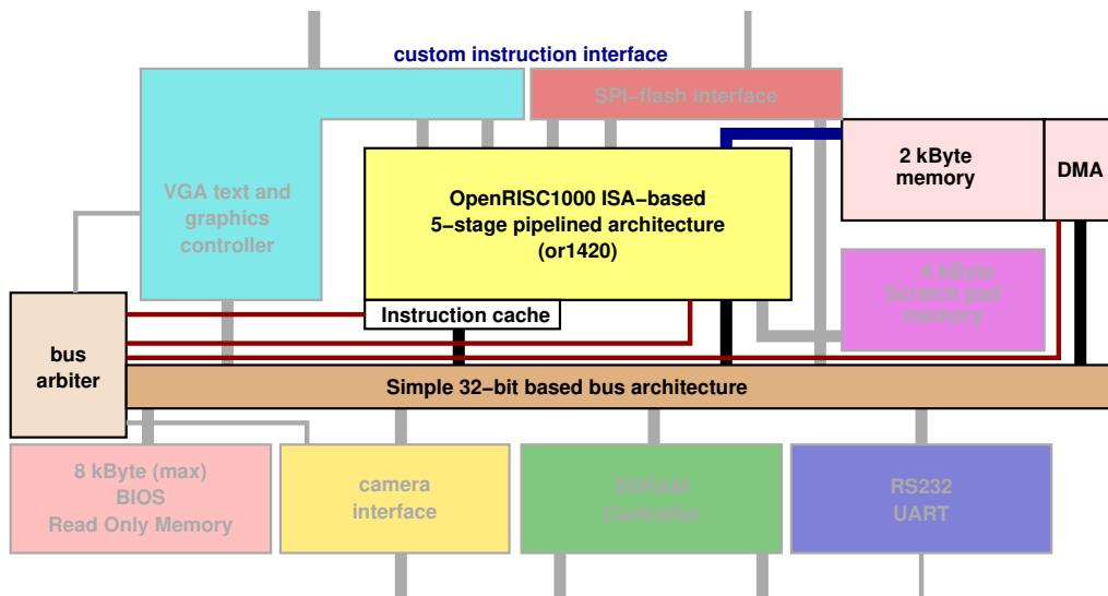
The DMA-controller is a master-device on the bus. For efficiency, the DMA-controller will support burst-mode.
