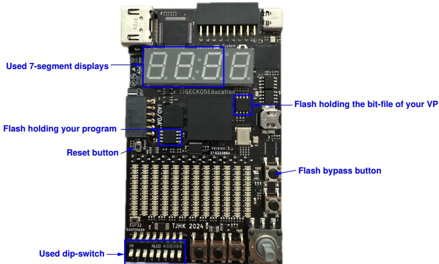
In the above picture you see the used elements. There are some nice features put in place to ease the usage of the platform:
