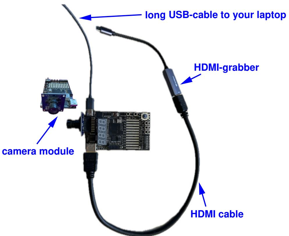
The HDMI-grabber will show itself as a webcam on your machine and the image can be shown by any program that can show the contents of a webcam.
