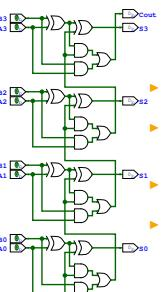
in this method we cut the circuit (critical path) in 2 (or more) parts.
