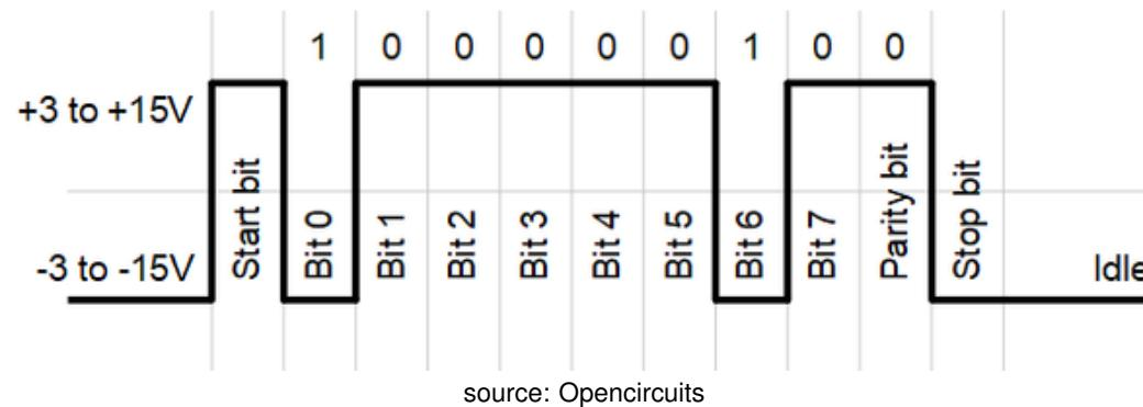
As the frame consist of 11 bits (containing one data byte), we can transfer a maximum of:
