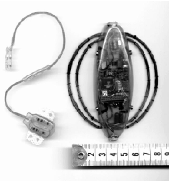
Fig. 12. Aalborg University implanted DFS implant and external unit. (Haugland et al. 2000, reproduced with permission.)
