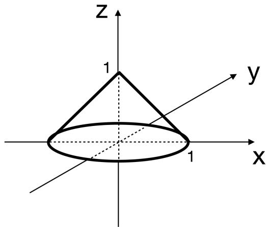
The image above shows a cone aligned with the z-axis. The apex (tip) of the cone is at  $(0,0,1)$ , the radius at the base in the  $xy$  plane is 1. We are also given a ray  $\mathbf{r}(t) = \mathbf{o} + t\mathbf{d}$ , where  $\mathbf{o} = (o_x, o_y, o_z)$  is the origin of the ray and  $\mathbf{d} = (d_x, d_y, d_z)$  is the ray direction with  $\|\mathbf{d}\| = 1$ .
