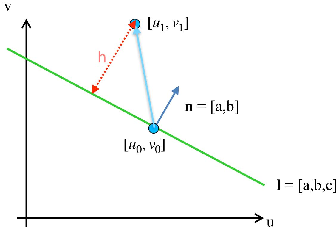
$$\begin{aligned}\text{Signed distance: } h &= \mathbf{n} \cdot [u_1 - u_0, v_1 - v_0] \\ &= a(u_1 - u_0) + b(v_1 - v_0) \\ &= au_1 + bv_1 - (au_0 - bv_0) \\ &= au_1 + bv_1 + c - (au_0 - bv_0 - c) \\ &= au_1 + bv_1 + c\end{aligned}$$
