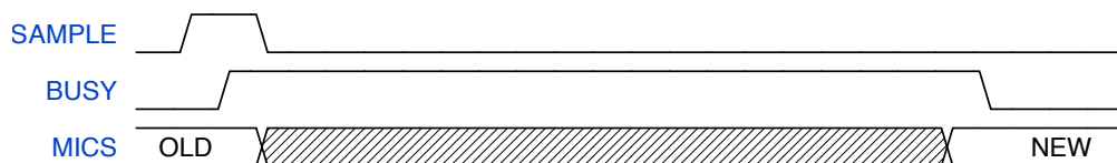
Figure 35: The timing diagram of the ADC.
