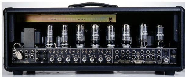
Their particular sound is mostly due to the distortion they introduce. That is, if the input signal is a sinusoid, the output will not be a perfect sinusoid but a distorted one.
