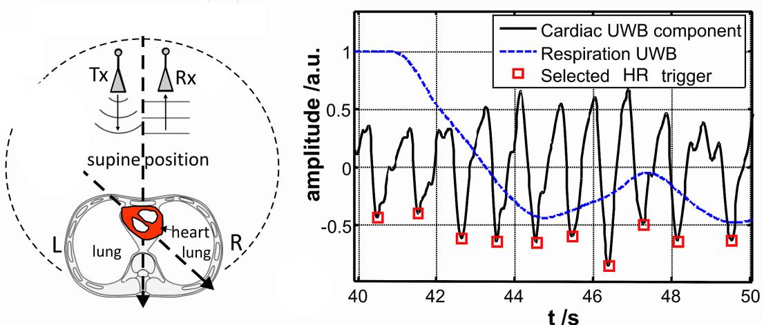
We suppose that the pulses are of very short duration and the they can be approximated to Dirac deltas. We call  $y(t)$  the received sequence of pulses, where  $y(t) = \sum_{n=1}^{\infty} \delta(t - \tau_n)$ , and  $\tau_n$ ,  $n = 1, \dots$  are the positions in time of the received pulses (Dirac deltas).
