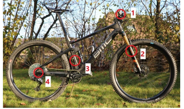
Fig. 2: Competition MTB with Sensor Positions.
