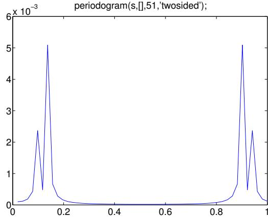
To be noticed that, being at the limit of spectral resolution, the line spectra do not appear to have the same amplitude!
