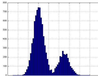
This suggests that the daily produced 10000 LED bulbs can be divided into two classes, each being described by a Gaussian distribution.
