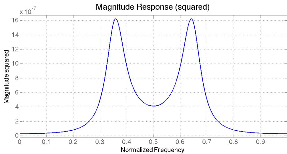
If the filter is considered anti-causal, then it is not stable and the transmittance evaluated on the unit circle (DTFT of the impulse response) does not exist.
