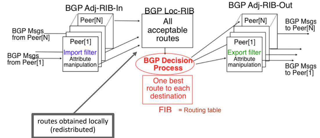
The result of the decision process is stored in forwarding table and in Adj-RIB-out (*one route per destination for each BGP peer*). The router sends updates when Adj-RIB-out *changes* (addition or deletion) after applying *export rules*.
