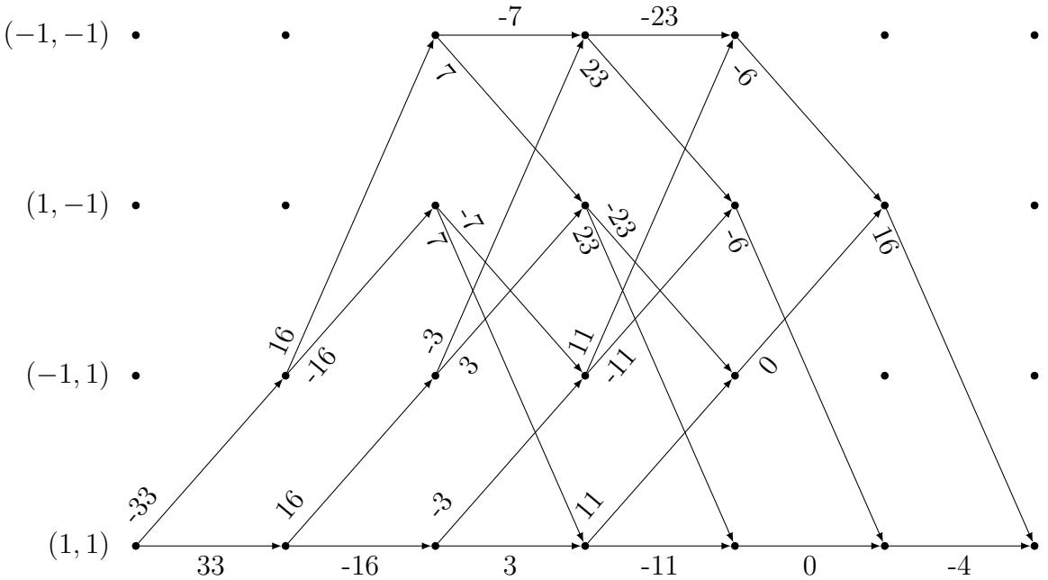
From the trellis, the channel metric is maximized if we choose input sequence  $\{1, -1, 1, 1\}$  with the path metric total of 72.
