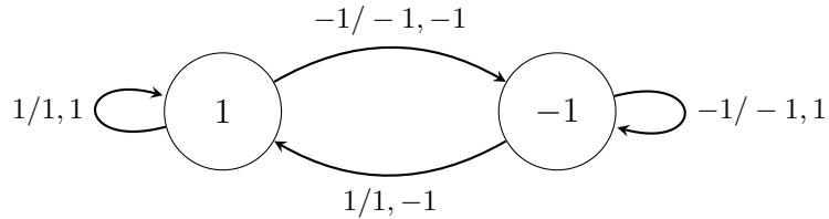
The circuit and state diagram corresponding to odd-indexed inputs  $d_i$  is identical to above. If the output of the odd-indexed inputs are  $\beta_{2i-1}\beta_{2i}$ , then the 4-state base encoder is obtained by interleaving outputs of the 2-state encoders as such:  $\alpha_1\alpha_2\beta_1\beta_2\alpha_3\alpha_4\beta_3\beta_4\dots$
