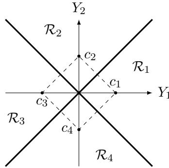
This is a 4-PSK constellation and the probability of error of an ML decoder for such a constellation is
