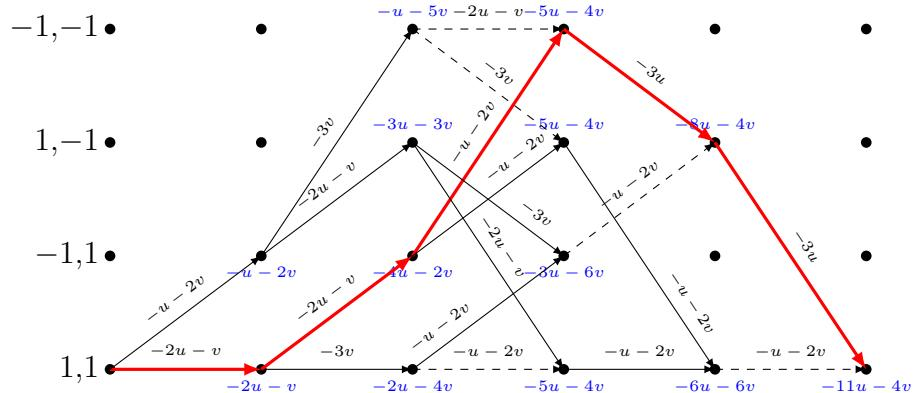
From the figure we can read the decoded sequence  $1, -1, -1, 1, 1$ .
