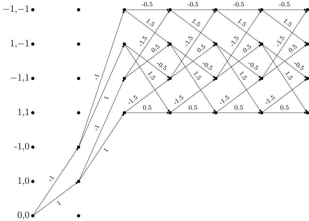
and the trellis labeled by the decoding metric,
