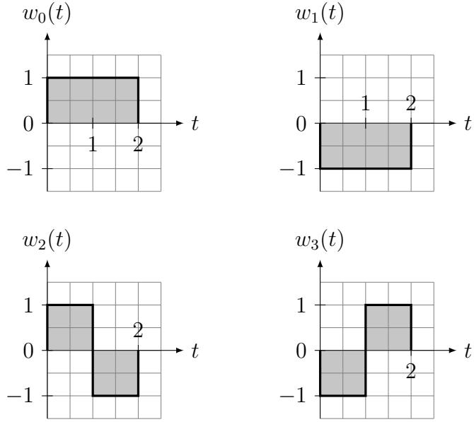
These waveforms are used to convey one of four messages over an AWGN channel with noise intensity  $\sigma^2$ . Assume that the four messages are equally likely.
