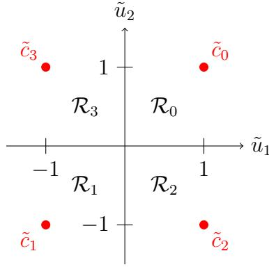
This is identical to the scenario in (a), as  $\tilde{c}_i = c_i$ , except that the variance is now twice. Hence, the error probabilities satisfy  $\tilde{p}_e(\sigma/\sqrt{2}) = p_e(\sigma)$ , and the desired ratio is 1.
