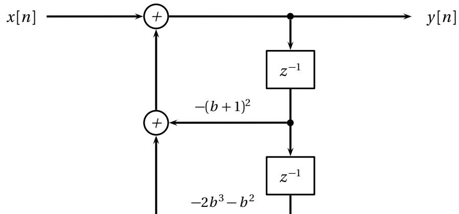
Alternately, since we already have the transfer function in factored form and since the two poles are real-valued, we can implement the system as a cascade of two first-order feedback loops as shown in the following figure; the advantage of this implementation is that it uses the actual values of the poles and therefore any potential issues due to limited numerical precision are mitigated.
