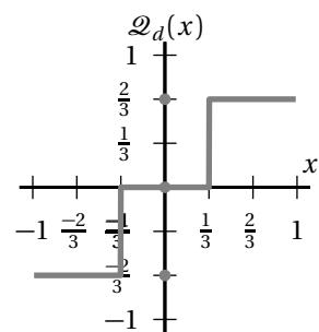
Both quantizers operate at two bits per sample but the deadzone quantizer "wastes" a fraction of a bit since it has only 3 quantization intervals instead of 4.
