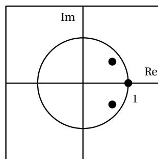
Select the only impulse response that is compatible with the given pole-zero plot. (For each impulse response, every value not shown in the plot is equal to zero.)
