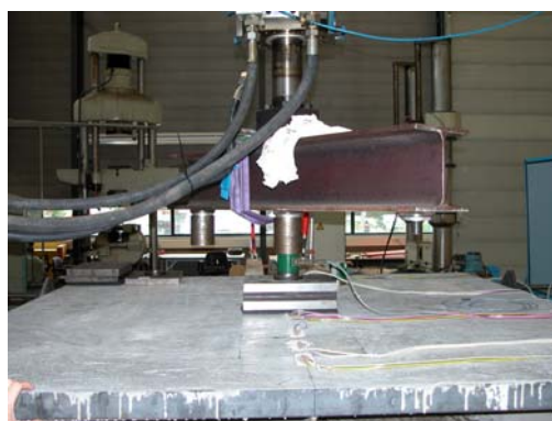
Photo 10: Testing RUHPC overlay on deckplate with fatigue cracks in TU Delft.
