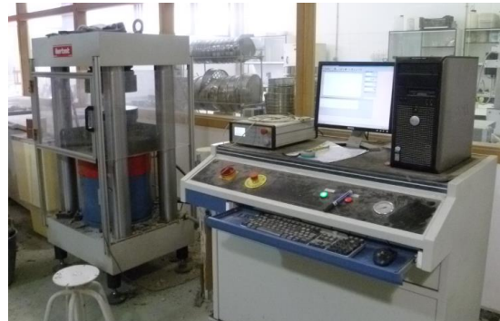
Figure 3.34: IBERTEST 3000 kN equipment
