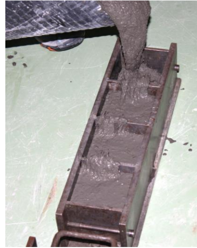
Figure 3.30: Prisms being filled
