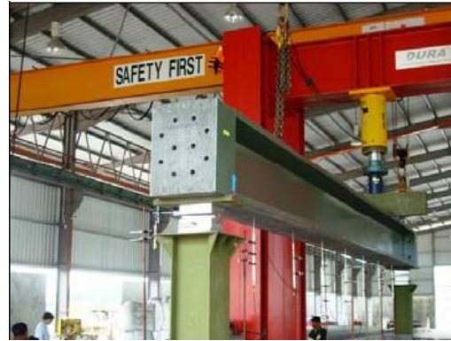
Figure 2.56: Shear test of a rafter beam, where the massive end can be seen
