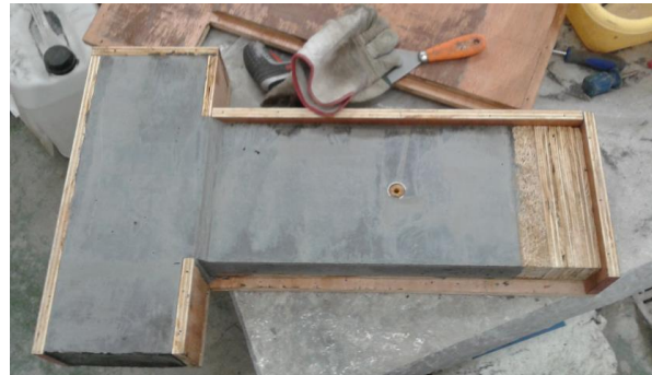
Figure 5.33: Element in the demoulding process
