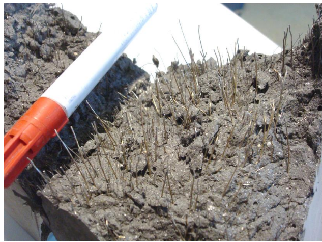
Figure 4.24: Flexural failure section opened, dosage F-6
