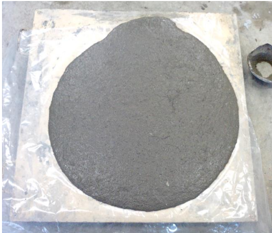
Figure 4.36: Slump-flow of CA-12
