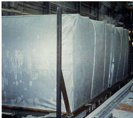
Figure 2.21: Wrapping of an element with polyethylene to apply the steam curing [20]
