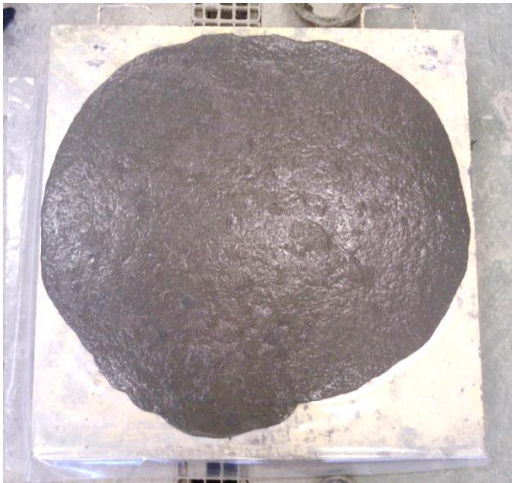
Figure 4.34: Slump-flow of CA-10
