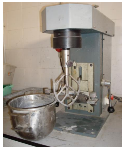
Figure 3.11: View of the mortar mixer
