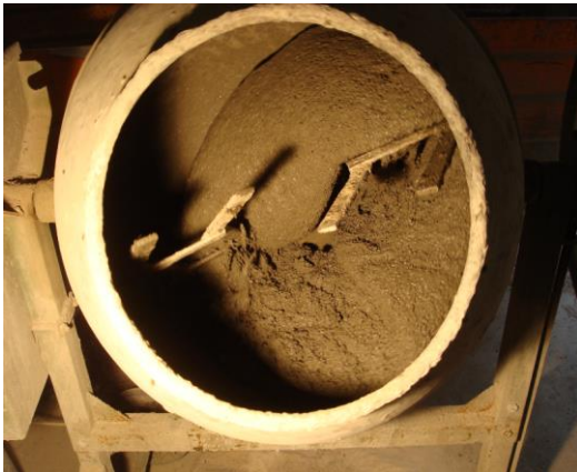
Figure 3.12: Drum mixer mixing UHPFRC
