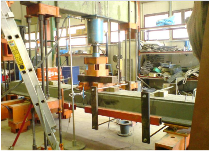
Figure 3.38: Bending test performed to a precast prestressed beam
