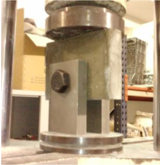
Figure 5.17: Bearing strength test set up
