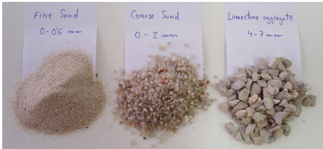
Figure 3.8: Photos of the quartz sand and limestone coarse aggregate
