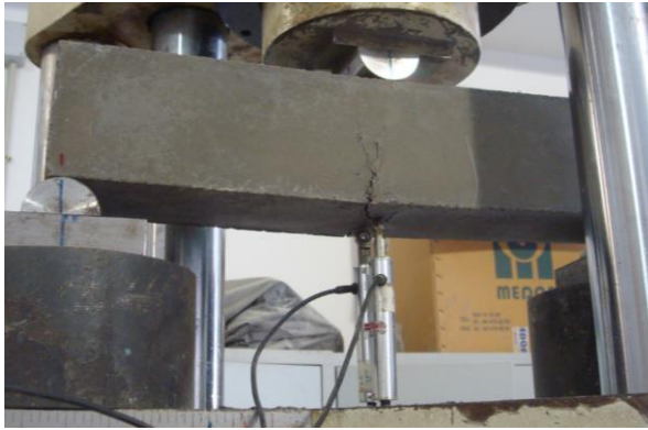
Figure 3.35: Three point bending test performed
