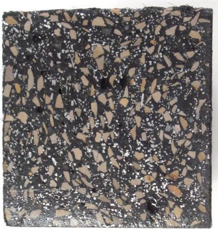
Figure 4.38: Cut section of a coarse aggregate prism
