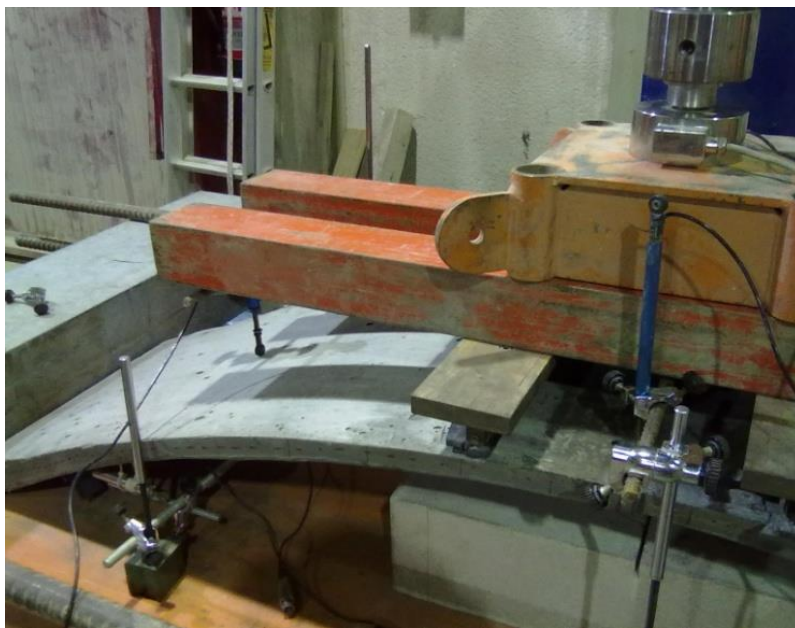
Figure A.10: Four point compressive test applied to the 30 mm thickness curved shell in laboratory
