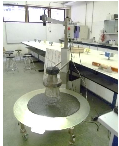
Figure 3.28: Rheometer developing a slump flow test
