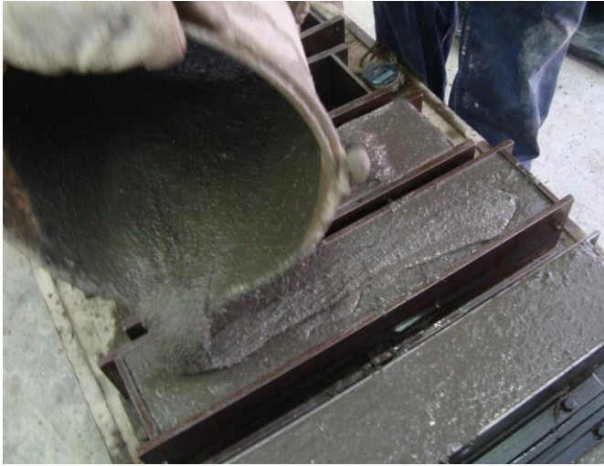
Figure 3.29: 100 x 100 x 400 mm prisms being filled
