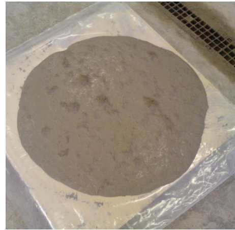
Figure 4.51: Slump-flow of dosage COM-3
