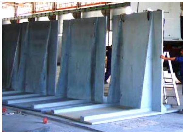
Figure 2.54: Retaining walls made with DURA®
