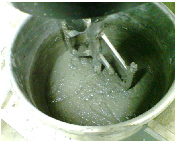
Figure 3.10: Mortar mixer with UHPC
