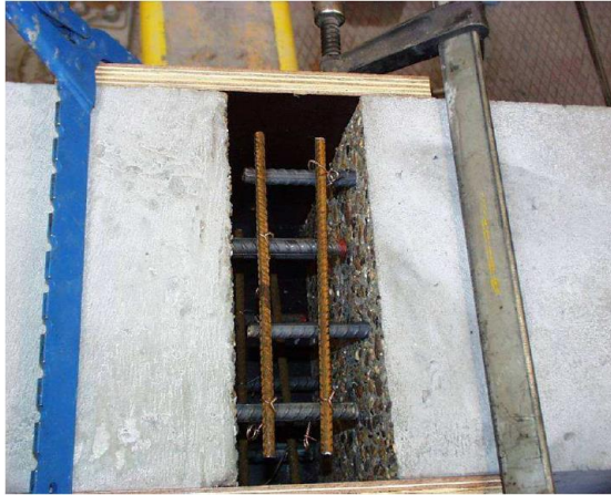
Figure 2.49: CRC joint made between OC elements
