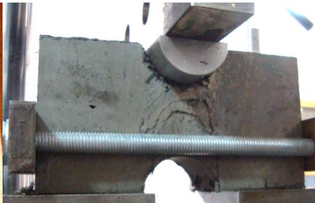
Figure 5.6: Bearing failure of a UHPFRC element
