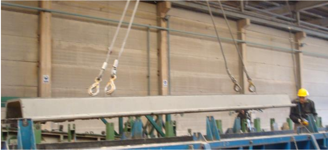
Figure A.4: Removal of a 5 meters length precast prestressed element 24 hours after casting
