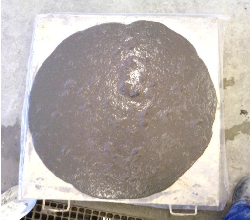
Figure 4.32: Slump-flow of CA-1
