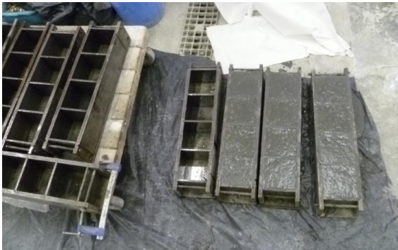
Figure 3.33: L=100 mm moulds
