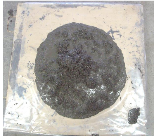
Figure 4.37: Slump-flow of CA-13
