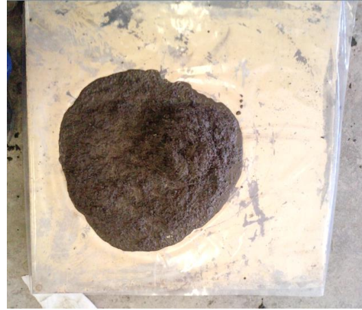
Figure 4.33: Slump-flow of CA-2
