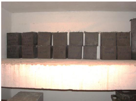
Figure 3.31: Cubes stored at 20^{\circ}\text{C}
