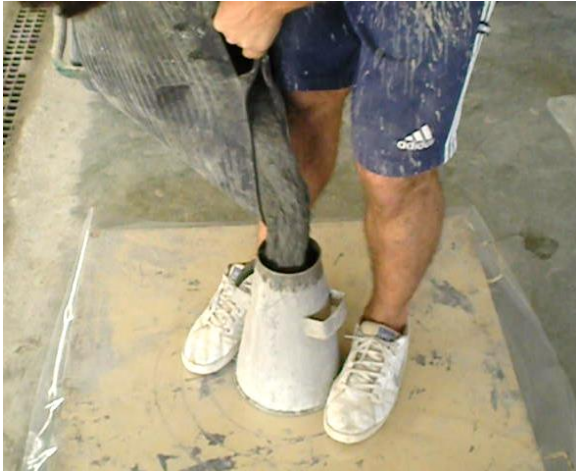
Figure 3.25: Filling of the cone with UHPFRC
