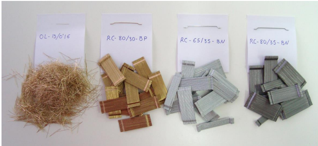
Figure 3.9: Photo of the different fibers used
