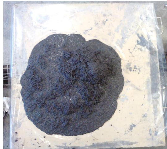
Figure 4.35: Slump-flow of CA-11
