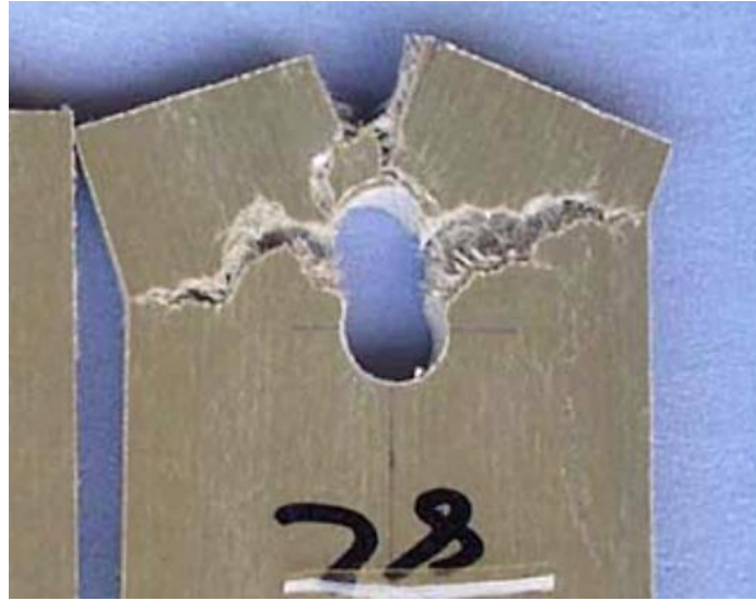
Figure 5.11: Cleavage failure of a pultruded GRP plate
