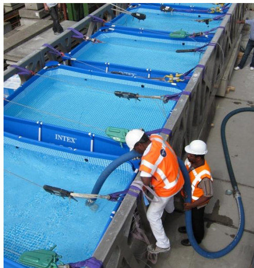
Figure 9: For the testing of the bridge, water containers were filled with water
