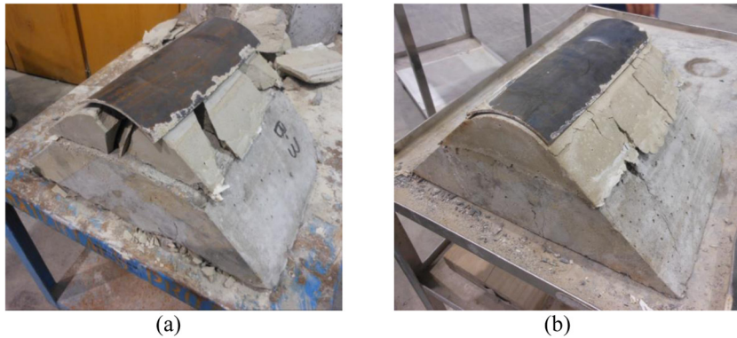
FIG. 6 Armor plate repair specimens following testing. Fiber reinforcement significantly reduced cracking and spallation of the repair material. (a) Non-fiber-reinforced specimen following testing. (b) Fiber-reinforced specimen following testing.
