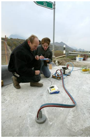
Figure 26: Air permeability measurements on a UHPFRC overlay cast on site and results
