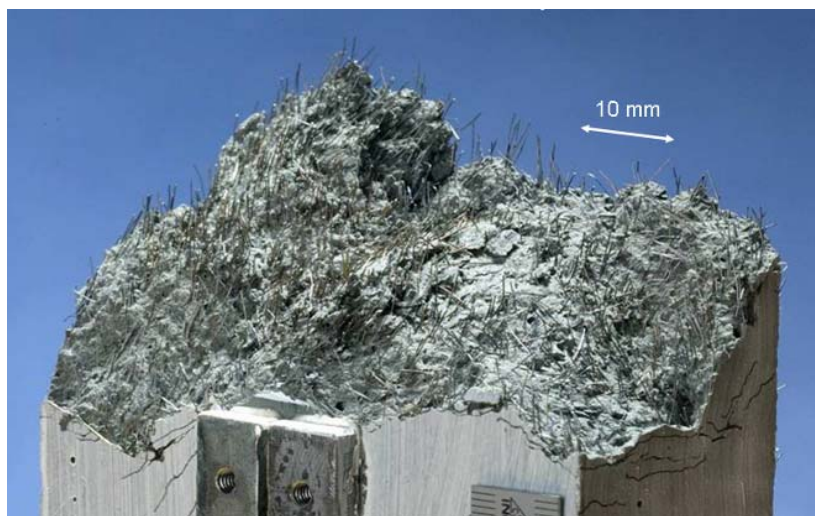
Figure 4: Fractured surface of a UHPFRC specimen, CEMTEC multiscale ®, recipe CM23.
