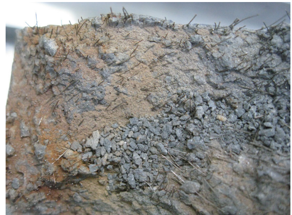
Fig. 12 Fracture surface showing matrix spalling and pulverization
