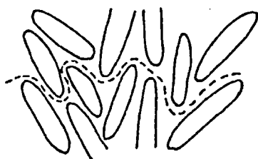
Fig. 8. Fracture mechanism in a xerogel such as hardened cement paste according to Higgins and Bailey (ref. 59).
