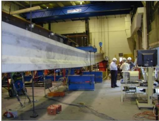
Figure 10. Photo. Flexural test of an AASHTO Type II girder made of UHPC
