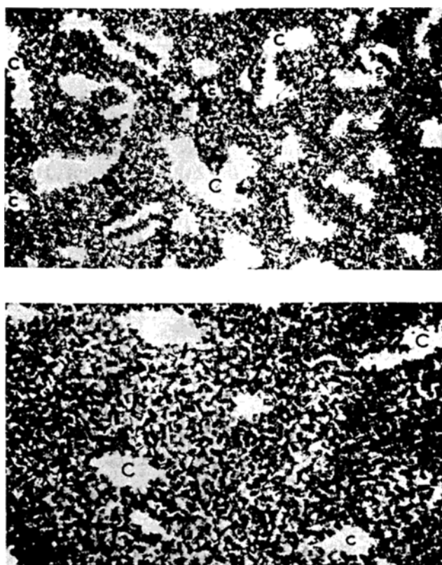
Fig. 4. — Simplified model of hardened Portland cement paste structure. Masses of randomly oriented groups of black lines represent cement gel. Spaces like those marked C represent mature paste. Upper drawing represents mature paste w_0/c = 0.5 , capillary porosity 20%; lower drawing represents nearly mature paste w_0/c = 0.3 , capillary porosity 7% [2].
