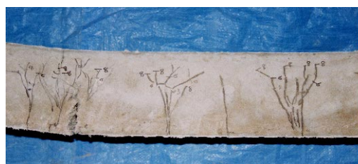
(b) ECC specimen without ribs
