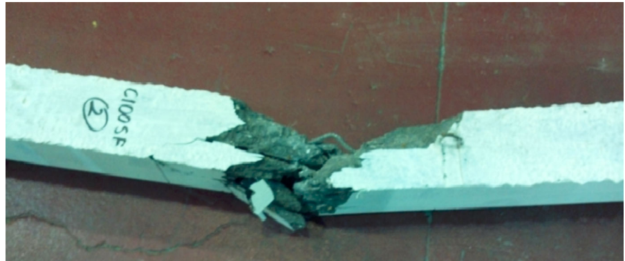
Fig. 26 Buckled C110 + 0.18 % SF column 2
