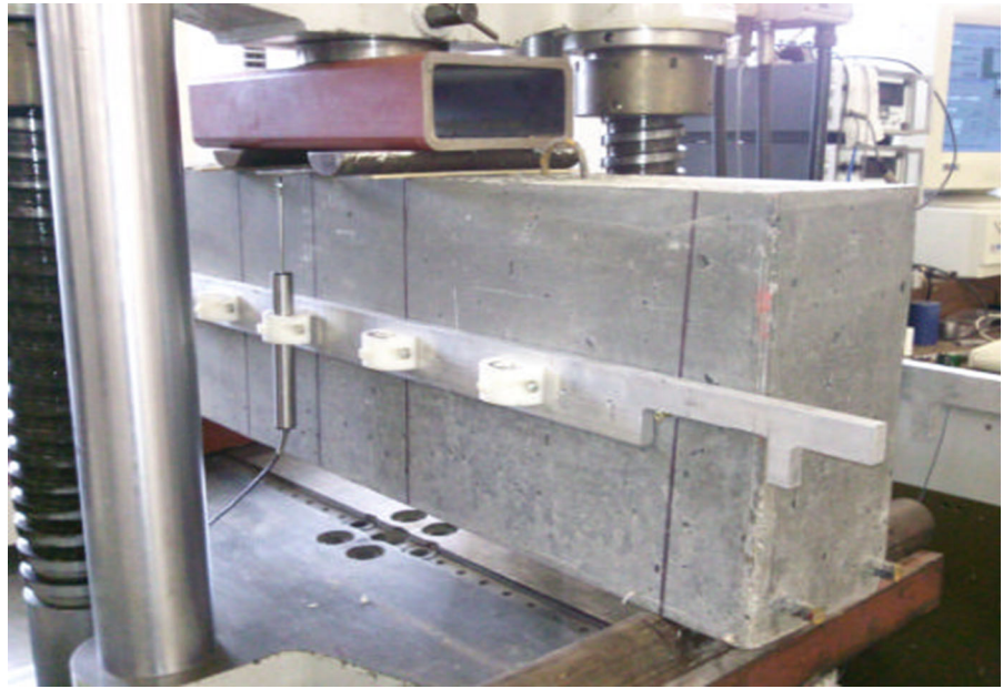
Fig. 17 Four point bending test set up of short beams over a span of 850 mm (span to depth ratio = 2.83)
