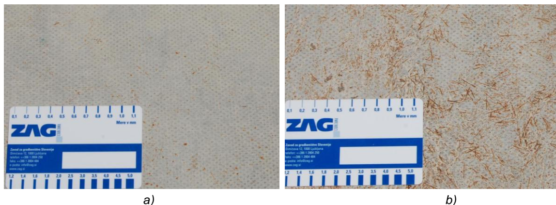
Figure 2: UHPFRC surface of excellent a) and poorer quality, with apparent fibres b).
