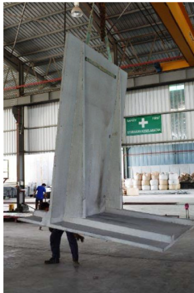
Figure 1. Precast UHPFRC 2.5 metre high retaining wall segment.
