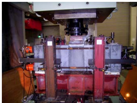
Photo 2 Loading test of UFC wet joint
