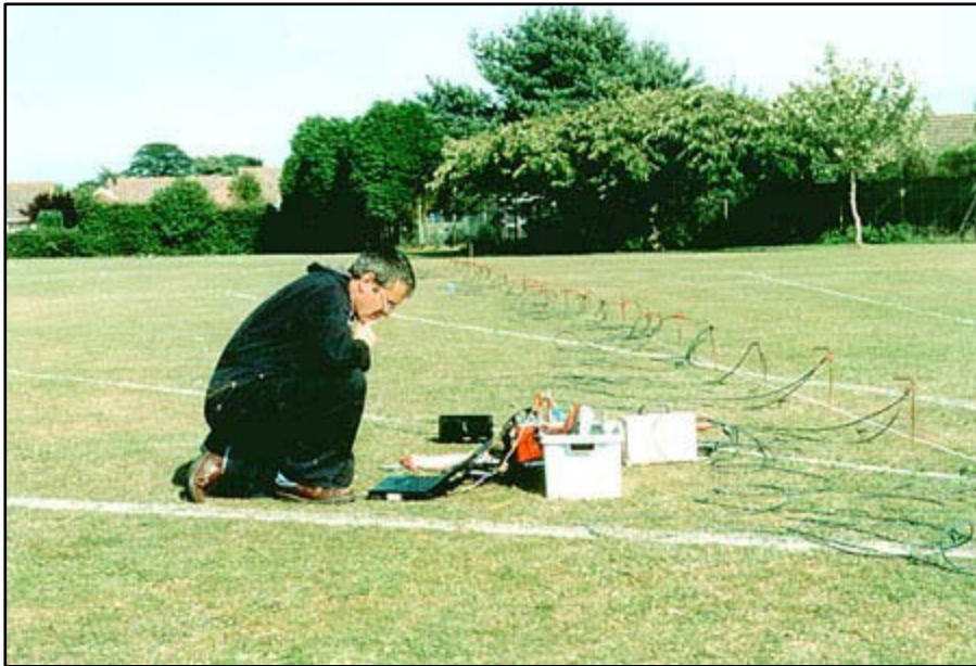
A multi electrode resistivity survey
