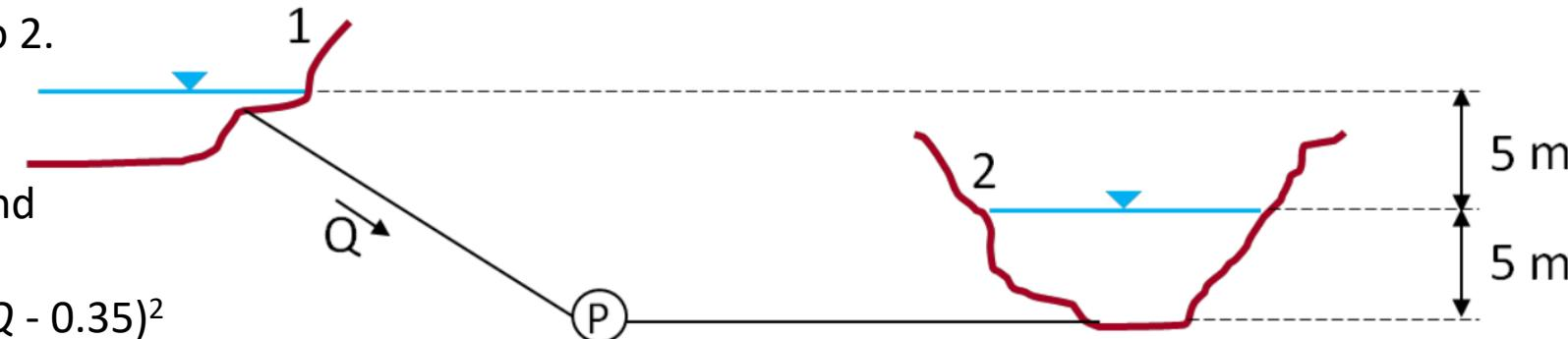
The pipeline has a total length  $L = 100$  m, and a diameter  $D = 0.25$  m. The pump is located halfway the pipeline.
