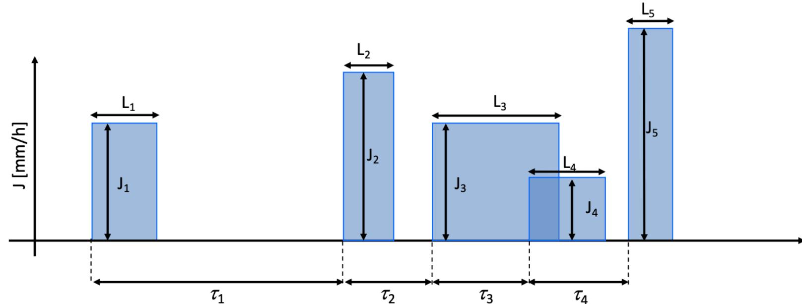
**Point model of rainfall. Continuous time model.** Occurrence of rainfall cells is modelled as a Poisson process. Each cell is characterized by a duration and a precipitation intensity. The process is described by **3 random variables**
