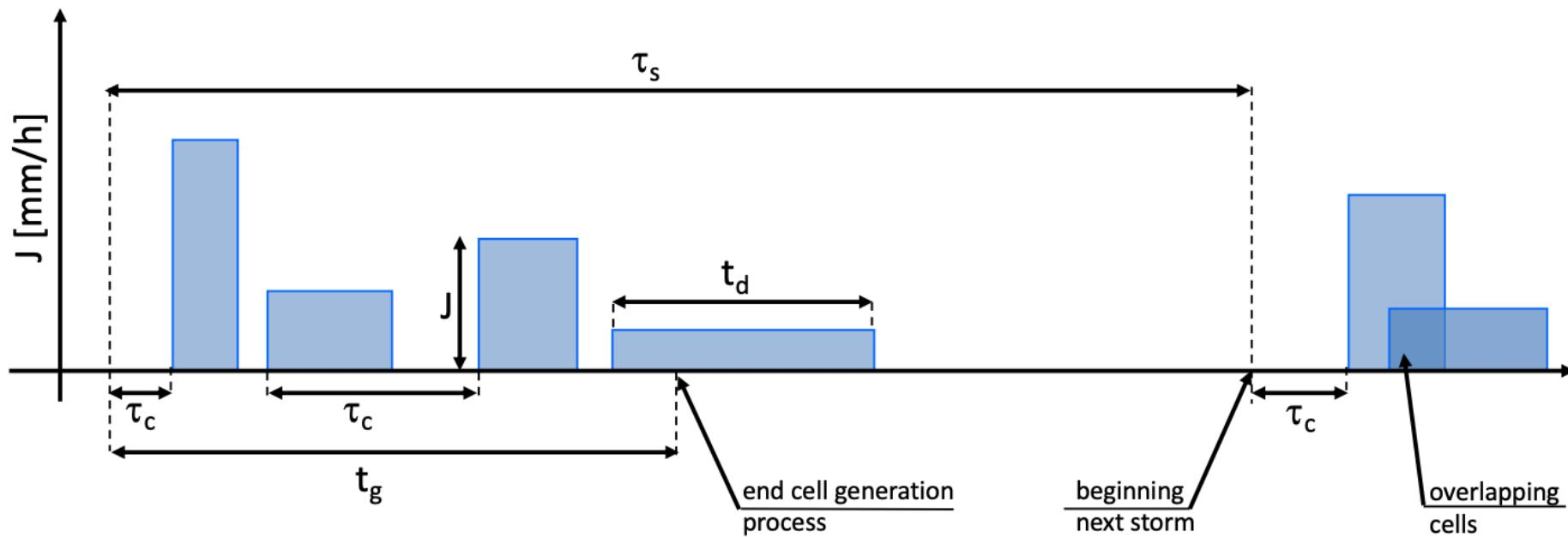
Point model of rainfall. Continuous time model. Rainfall occurs in storms characterized by a certain duration. Within each storm, rainfall cells are generated as in the rectangular pulse model. The process is described by 5 random variables generically assumed exponentially distributed
