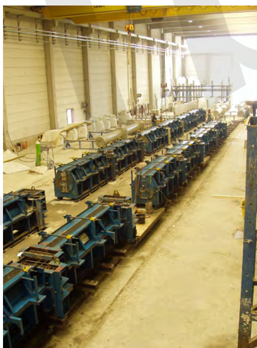
Fig. 6-18: A family of moulds set up for horizontally casting double storey circular columns with intermediate corbels. Note the finished column alongside the mould in the background (courtesy of Ergon Structural Concrete).
