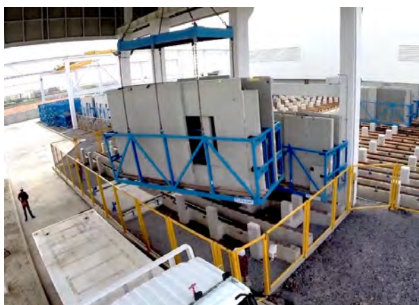
Fig. 7-22: Wall panels in steel racks being loaded onto a delivery vehicle (courtesy of Progress Group).
