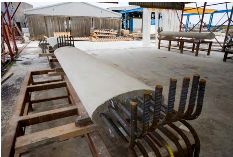
Fig. 6-1: Elliptical cross section with projecting top connection bars.
