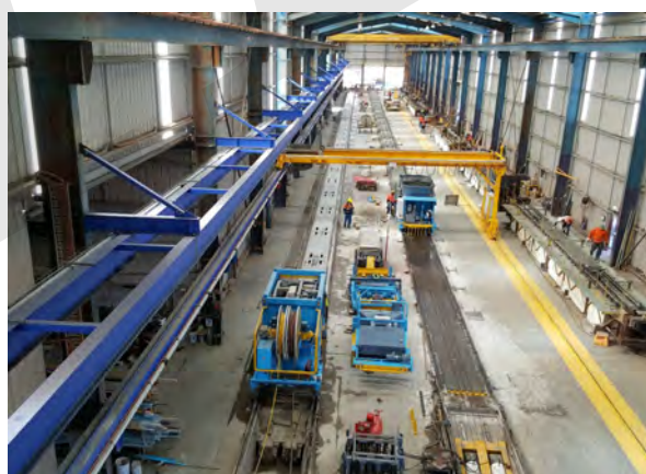
Fig. 5-15: Long line hollowcore production.
