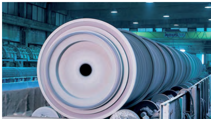
Fig. 6-21: Spinning formwork / machinery for precast concrete columns.
