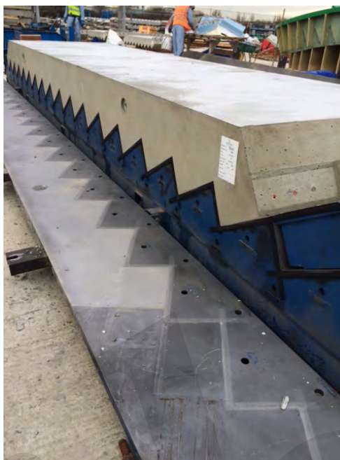
Fig. 8-17: Linear flight cast “face downwards”.
