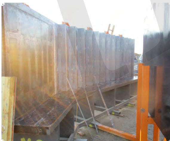
Fig. 8-18: Example of “on edge” mould.
