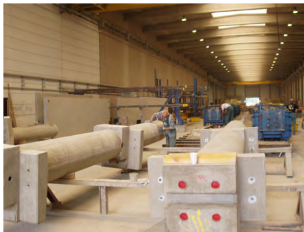
Fig. 6-19: Finishing double storey columns at the factory.
