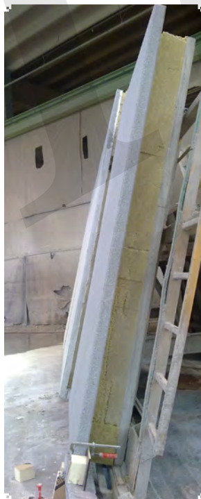
Fig. 9-4: Example of insulated sandwich panel from Finland.
