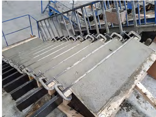
Fig. 8-21: Ramp mould after concrete placed.
