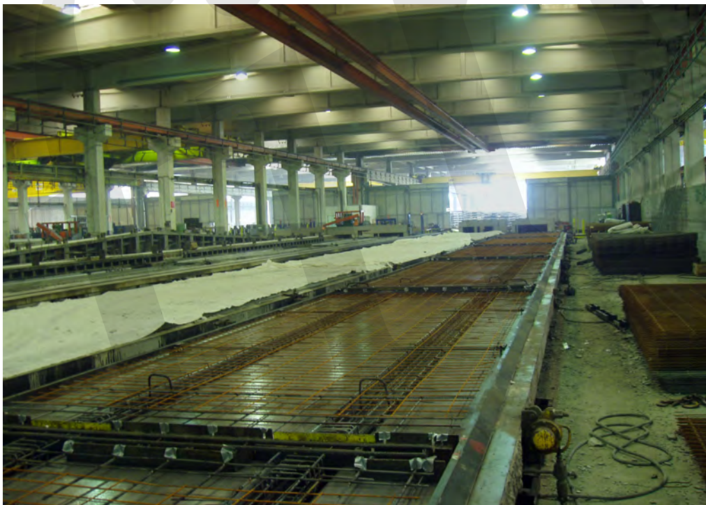
Fig. 2-10: Long line slab bed in precast factory.
