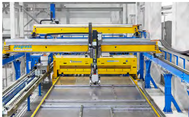
Fig. 7-27: Shuttering robot (courtesy of Progress Group).
