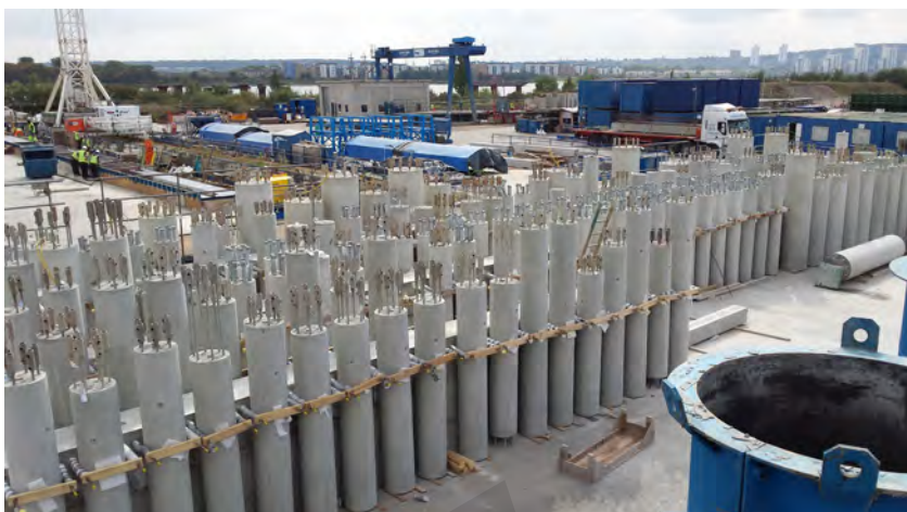
Fig. 6-16: Circular columns in the storage yard awaiting despatch (note the steel mould in the foreground).
