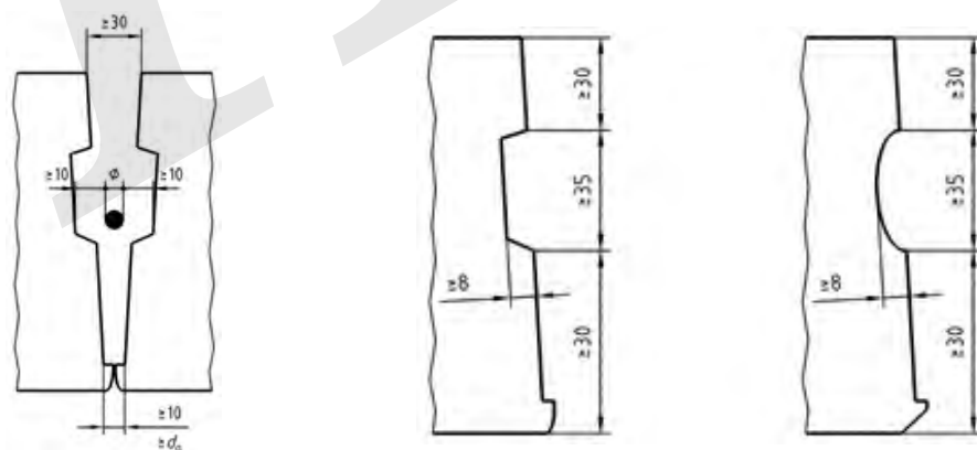
Fig. 5-32: Examples of edge profiles used mainly for vertical shear transfer.
