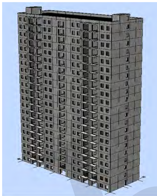
Fig. 2-4: Elevation of precast concrete cellular building.
