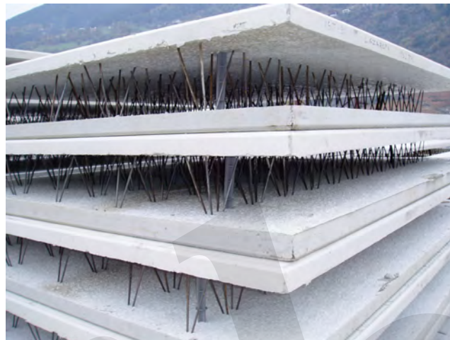
Fig. 7-20: Horizontally stored twin wall panels.
