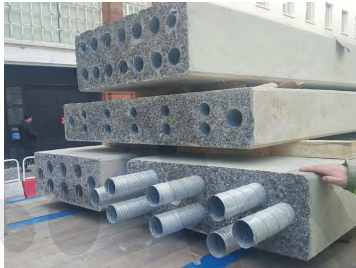
Fig. 6-15: Simple rectangular sections with cast in tubes for connection.
