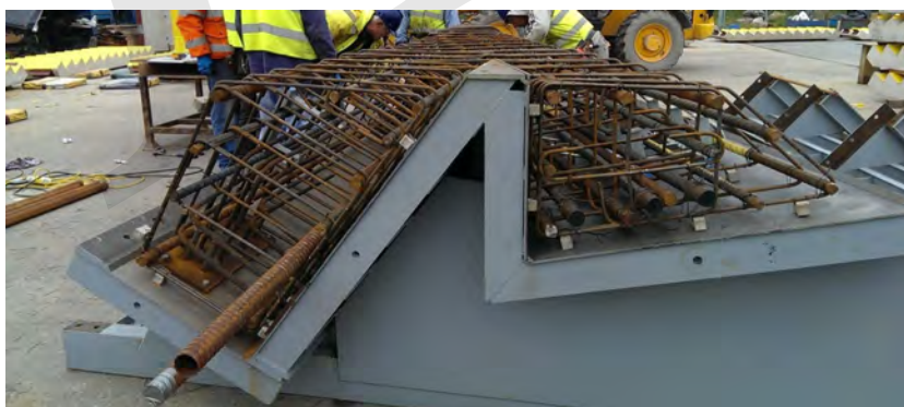
Fig. 6-14: Steel mould for non uniform shaped column.
