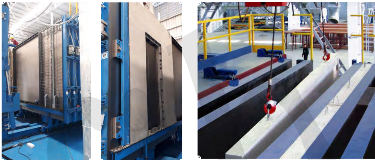
Fig. 7-23: : Battery mould process from preparation through to demoulding.
