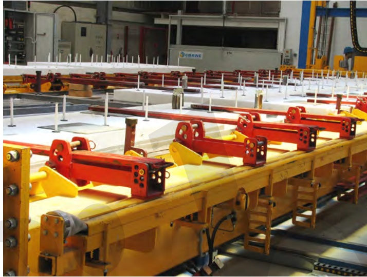
Fig. 7-33: Turning device for insulated twin wall panels.
