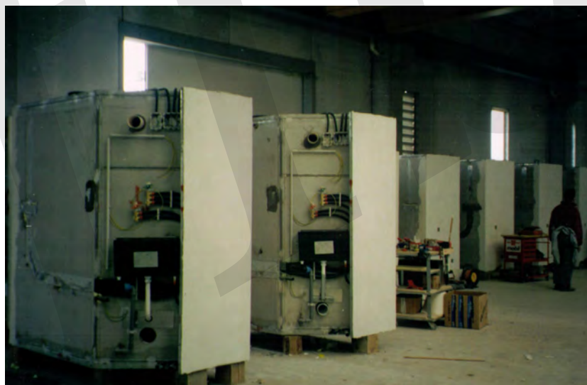
Fig. 3-19: “Plug and Play” bathroom pods assembled in factory conditions.
