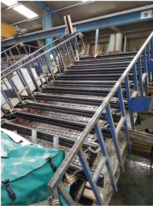
Fig. 8-20: Ramp mould prepared to receive concrete.
