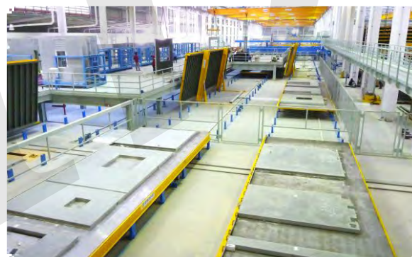
Fig. 7-25: Circulation factory with tilting tables at end of process and panels stored in racks.
