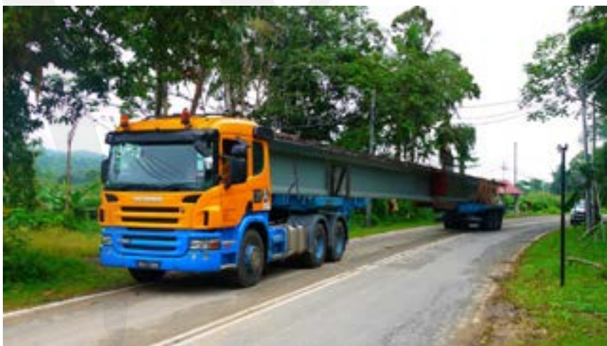
Fig. 5-186 Example of Transporting a decked T girder by truck and trailer.
