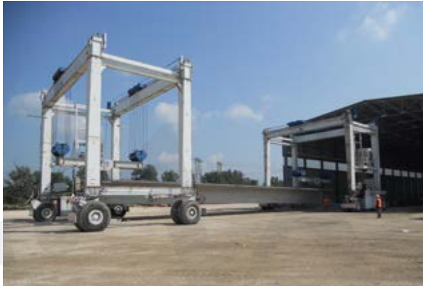
Fig. 5-121 Moving the girder from the precasting area of the factory to the storage lot.
