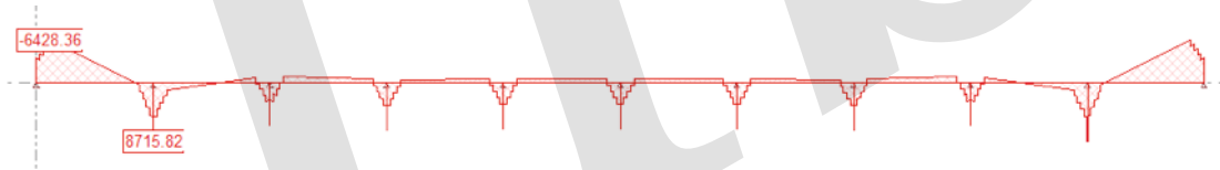
Fig. 9-9 Bending moment distribution due to prestressing
