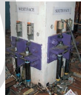
Fig. 5-59 Internal vs. external replaceable dissipaters/fuses at the base-column/pier connection (based on Marriott et al., 2008; NZCS, 2010)
