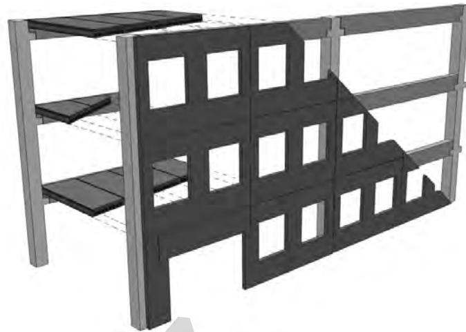
Fig.2.19: Outline of façade with non-load-bearing, precast-concrete cladding
