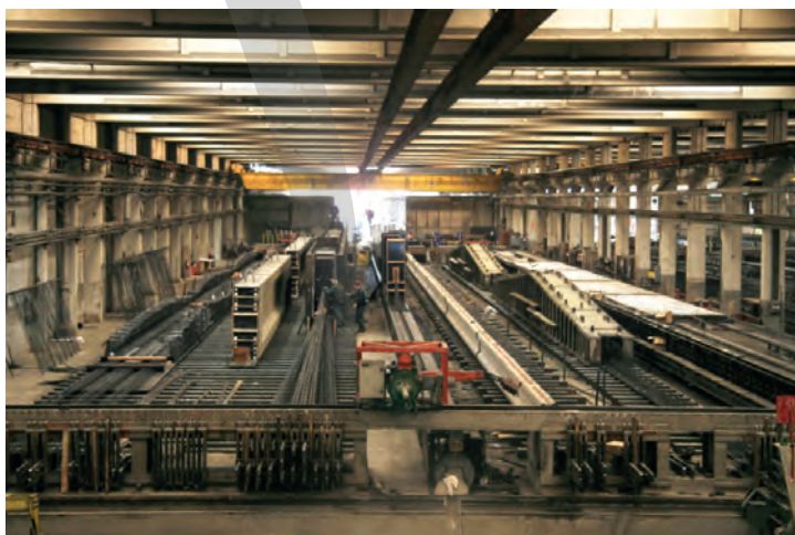
Fig. 1.8: Prestressing methods use long-line casting beds of between 100-150 metres in length
