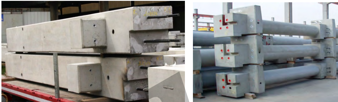
Fig. 6.27: Precast columns with rectangular and circular cross section. The sleeves in the top of the circular columns are used for the continuity of the peripheral tie bars around the corners of the building. The vertical tie bars in the corbels are fixed in anchored sockets.
