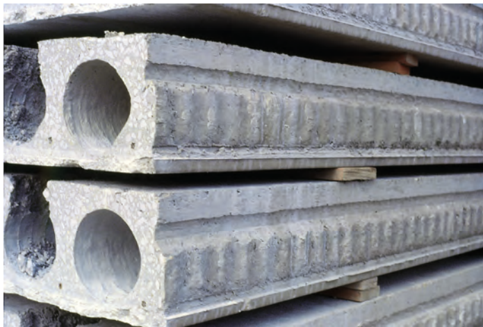
Figure 4.14: Longitudinal joints of hollow-core slabs with waved shear key. The behaviour of the slab-to-beam joints is also relevant. Special attention should be given to the anchorage of the slabs' longitudinal reinforcement into the beams.
