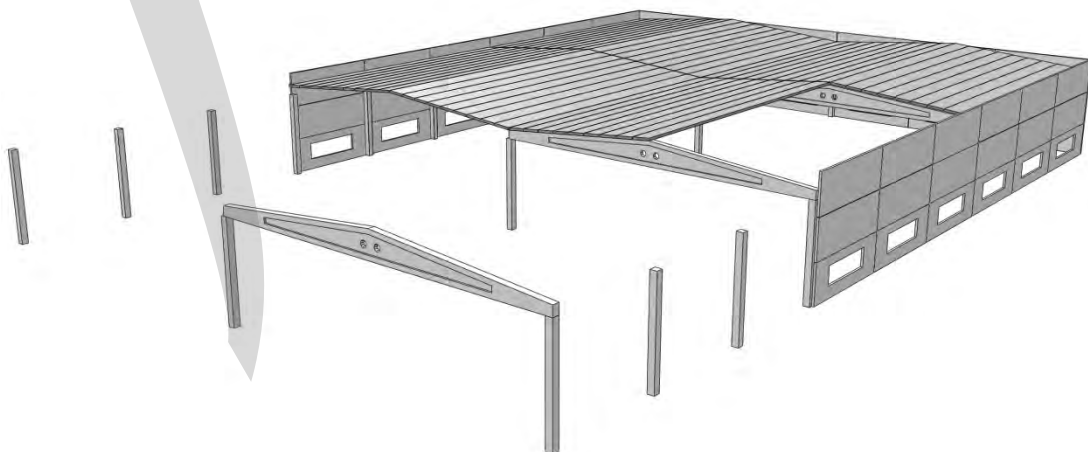
Fig. 3.16: Scheme of an industrial building with portal frames and ribbed concrete roof units
