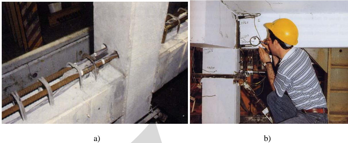
Fig. 9-16: Beam end to column connection, a) continuity of tie steel passing through sleeves in columns, b) measurement of beam-column rotation provides the data to determine semi-rigidity of the connection.
