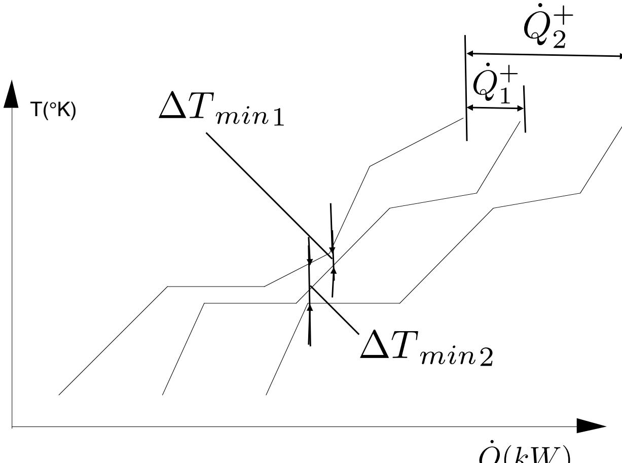
$\Delta T_{min} 1 < \Delta T_{min} 2$
