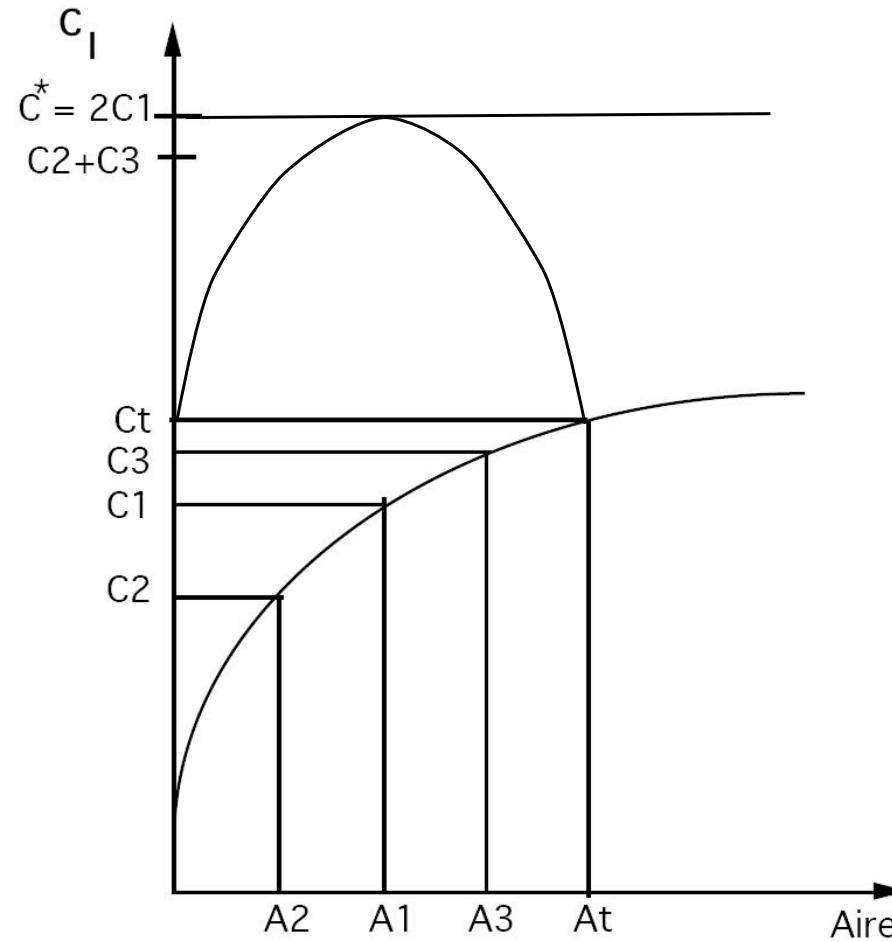
by assuming an equal repartition of the area over all the heat exchangers, we will overestimate the heat exchangers total cost.
