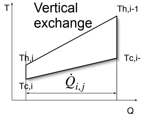
$$A_i = \frac{1}{(\Delta T_{lm})_i} * \left( \sum_{j=1}^{(n_{streams})_i} * \left( \frac{\dot{Q}_{i,j}}{h_{i,j}} \right) \right)$$
