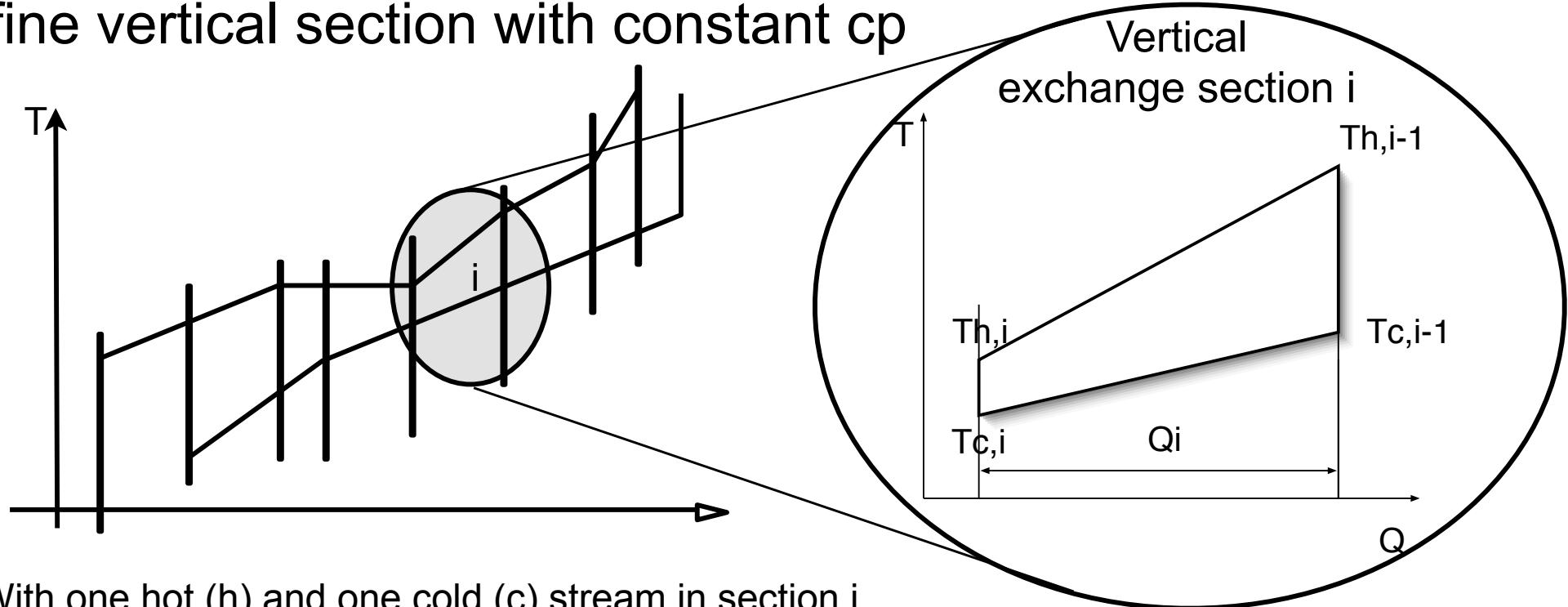
With one hot (h) and one cold (c) stream in section i
