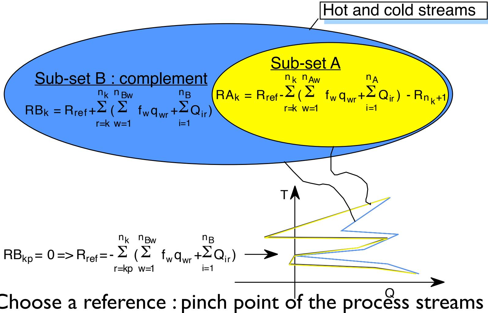
The integrated composite curve represent the way a sub-system is integrated with the remaining system.
