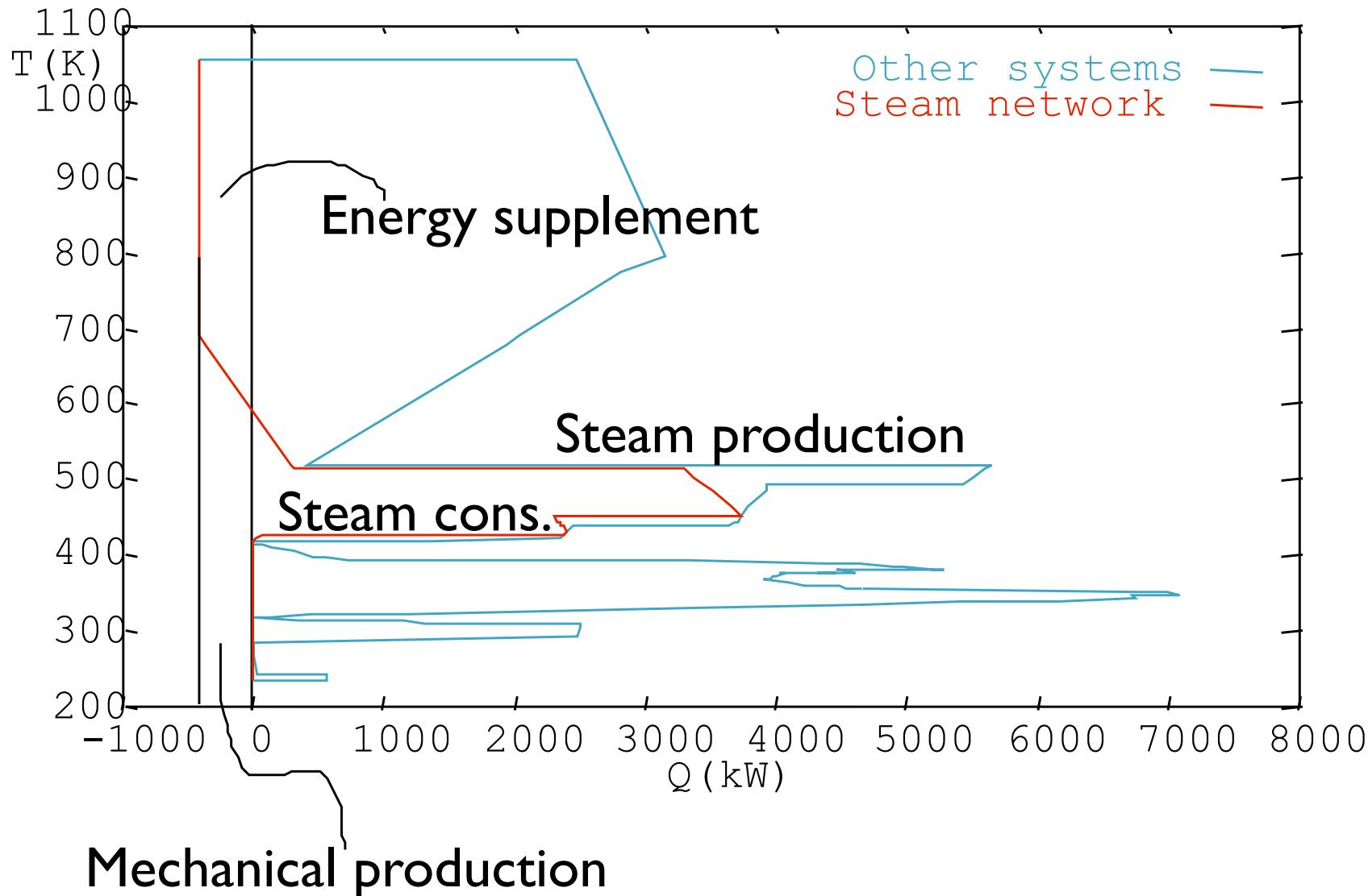
Note that for a closed cycle like refrigeration or Rankine, the sum the hot stream - the sum of the cold stream is the net mechanical power (i.e. the distance between the two extreme points is equal to the mechanical power). Here for the steam cycle. Note that it is therefore easy to verify that the cogeneration cycle is well located wrt the pinch point.
