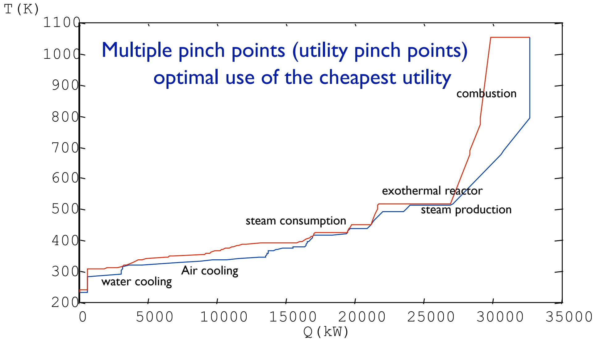
The balanced composite curves include the process and the utility streams. The balance is now closed has no magic hot or cold utility is used.
