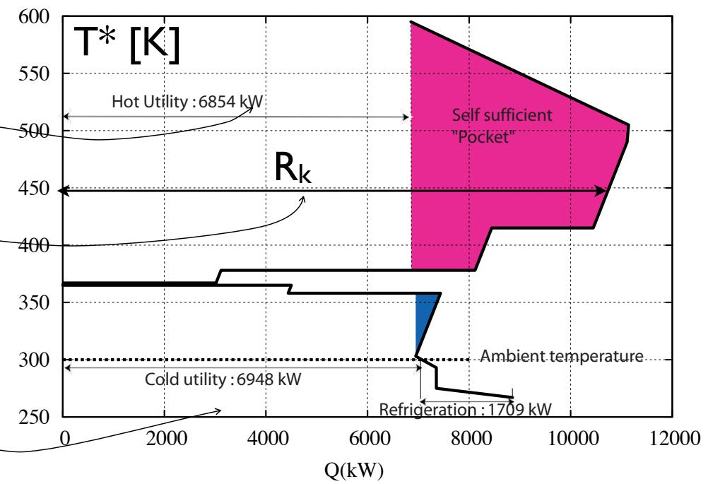
The Grand composite is the heat cascade representation in the corrected temperature domain. It represents the flow of energy in the system from higher temperatures to lower temperature. Above the pinch point is also represents the heat-temperature profile of the heat to be supplied to the system and below the pinch it represents the heat-temperature profile of the heat available in the process and to be removed from the system.
