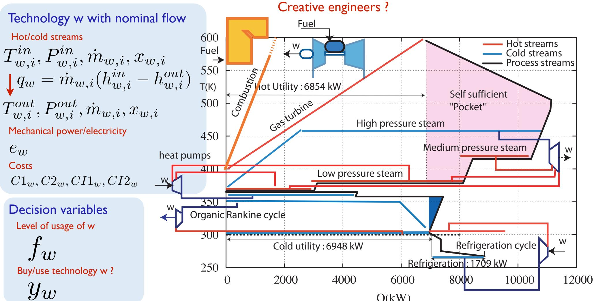
by simulation we can generate the hot and cold streams associated to a predefined level of usage (or flow).
