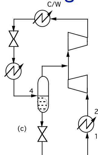
Two stages with intermediate cooling (system integration)
