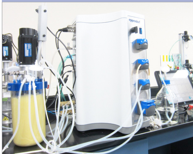
Figure 8: High-density E. coli culture in the BioBLU 3f Single-Use Vessel. Fed batch fermentation process 11 hours post inoculation
